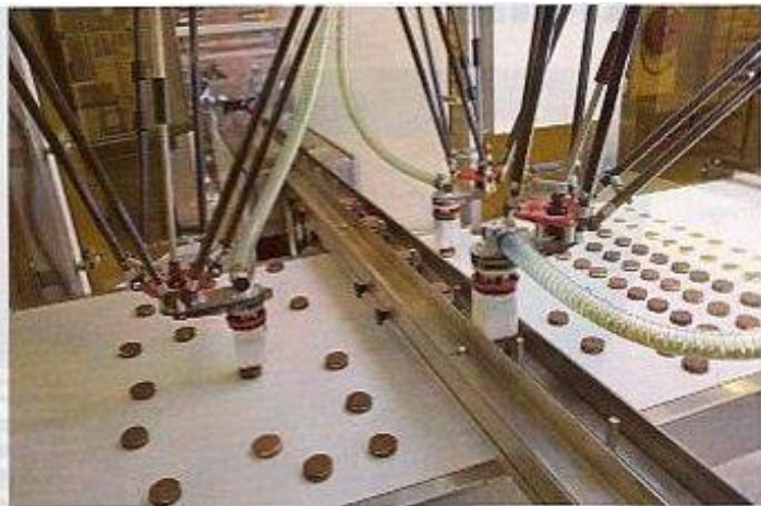
FIGURE 2. Single-camera solutions, such as this cookie packing system from Bosch Packaging Technology, use a geometric pattern-matching algorithm to determine the shape and location of cookies and then stack them in the appropriate section of the tray
