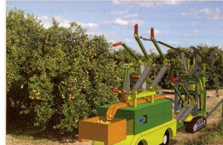
FIGURE 3. To automate the process of orange picking, Vision Robotics has proposed the development of a stereo camera-based system that will use multiple cameras placed at the end of multiaxis arms to create a virtual 3-D image of the entire orange tree.
